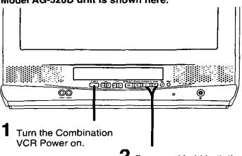
2 Press and hold both the PLAY and FF on the Combination VCR for more than 5 seconds.
